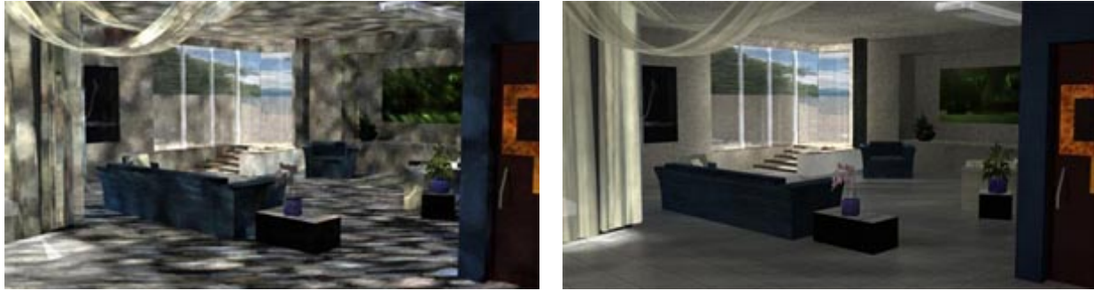
Figure 3. The top image was rendered with one non-photon generating infinite light (used for creating sunlight shadows and 2 spot lights generating 70,000 global illumination photons with a GI accuracy setting of 400, a photon search radius of 1.1, a combined trace depth on each light of 20, and Gauss filtering. This lower setting is useful to make sure that GI is functioning within the scene and that your photons are covering the space evenly, prior to increasing them for final render quality. The lower image shows the room with higher global illumination sampling applied. It has each spot generating 150,000 GI photons with a GI accuracy setting of 550, a photon search radius of 6, a combined trace depth of 24, and Mitchell filtering. It also has ambient occlusion applied to the walls, curtains, and furniture so the scene is noticeably smoother.
