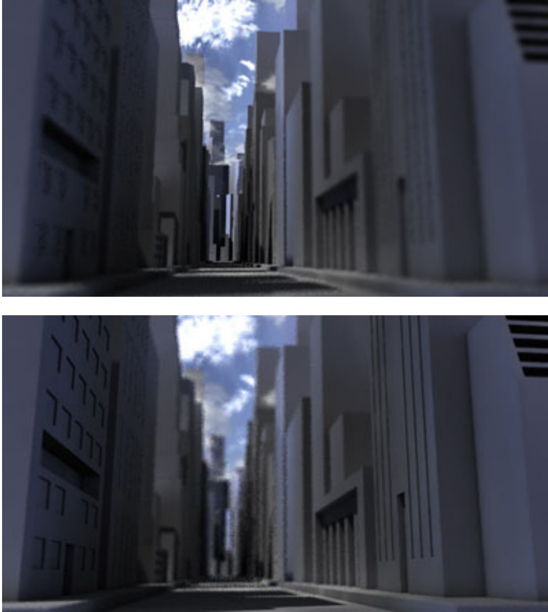
Fig 8. In the top image, A) a lens with a focal length of 80mm is used at f32, with a narrow circle of confusion (0.1), and a focal distance of 70. In the second image, B) the lens is still an 80mm, but the F-stop setting has been changed to f2. In both cases, the Depth of Field Strength is set at 0.07. To animate this effect, one would simply set keys on the focal distance and F-stop in frame 1 using the first values, and then advance the timeline to frame 60 and set another key with the second set of values, thereby creating a 2 second rack focus effect at 30 frames per second (fps).
